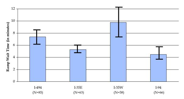
Figure 6.11 Average Ramp Wait Times Among Metered Users "With Ramp Meters" Corridor Surveys
