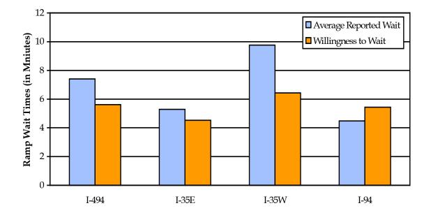
Figure 6.13 Maximum Willingness to Wait at a Ramp "With Ramp Meters" Corridor Surveys (N=507)
