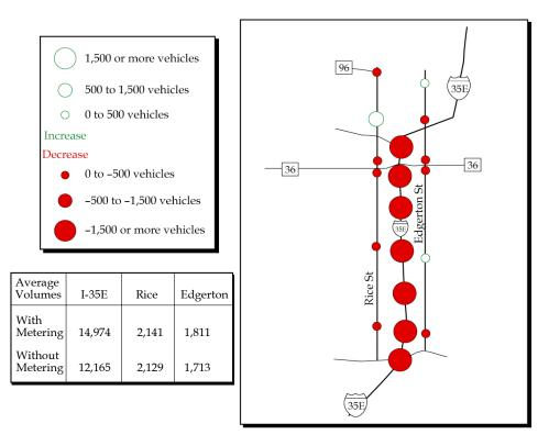
Figure 5.19 I-35E SB A.M. Traffic Volume Differences
