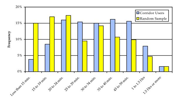
Figure 6.7 Freeway Travel Times - "With Ramp Meters" Surveys
