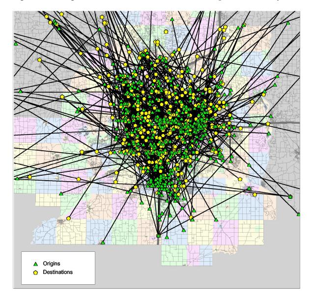
Figure 6.5 Origin-Destination Patterns – "Without Ramp Meters" Surveys
