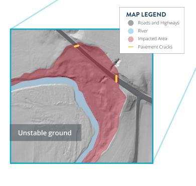
The illustration below highlights findings of this analysis – a lot of the ground underneath the roadway is unstable. Repairing the roadway in place would require significant specialized construction to stabilize the ground.
