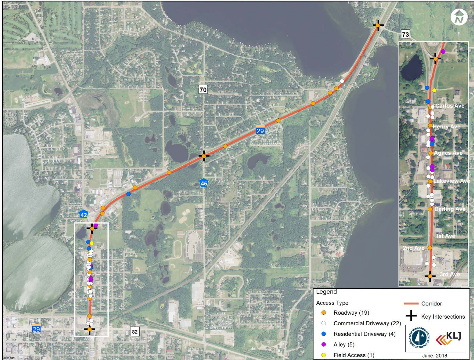
Figure 2.4: Access Locations on TH 29
